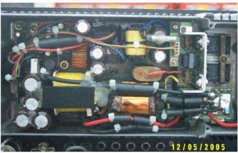
[The repaired and re-installed board; there is an added 3.15 amp fuse in the 280V input line; R2 was replaced with a high quality sealed multi-turn pot mounted on one of the 33V line electrolytics].
