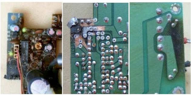
Burned PCB and copper traces near the R32, Q7 and R26; some parts are missing here.
