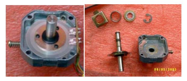
Clean the dirty shaft and the sleeve bearing remove the existing grease using isopropyl alcohol and then re-lubricate shaft and bearing. To reduce any backlash, lubricate with grease rather than oil. Don't use much grease; a small quantity will suffice. Avoid getting lubricant on the optical parts;
