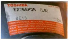
The CRTs are vacuum tubes, so they are actually "consumables". This is true not only for the cathode system (regarding its electron emission capability) but also for the CRT's screen surface phosphor. The burns are the result of the "consumable" phosphor. As the sum of these two characteristics, the CRT's brightness, contrast and focus quality may get low after extended use. This is why the allowed CRT brightness and contrast will be reduced after extended use.
