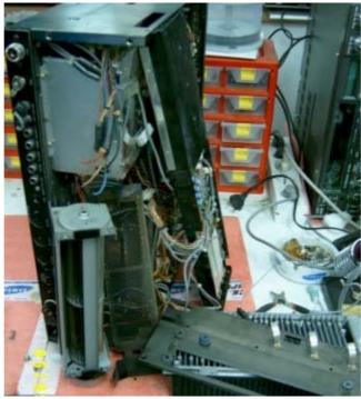
IC-781; heatsink and fan removed;
